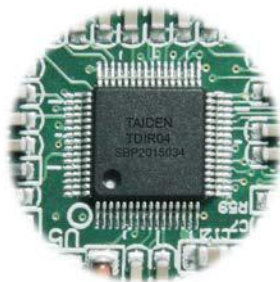
Figure 1 TAIDEN TDIR04 digital infrared processing chip
